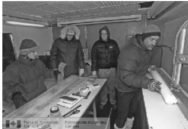
Glaciology research scientists from the Geological Survey of Canada are cutting samples from the Mount Logan core in the cold room lab in Ottawa.
