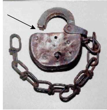
Figure 10 - Damaged switch lock. Note broken clasp mechanism (arrow)
