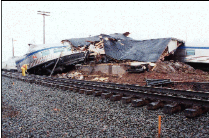
Figure 2 - Damage to diner car and farm supply building. Note foundation wall and roof of building in centre of photograph.
