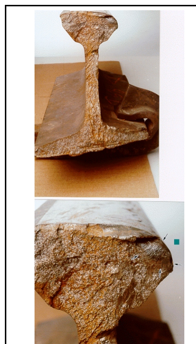
Figure 3 - Transverse defect representing three per cent of the rail fracture surface area.
