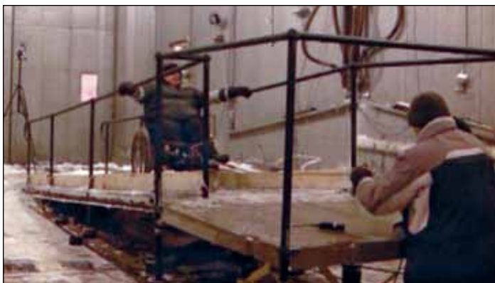
Figure 1 Ramp ascent on ice-grit using handrails
