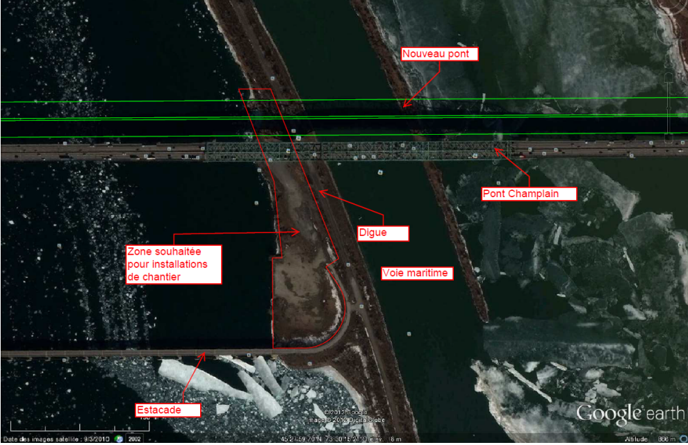
Figure 4 Jobsite location – Dike
