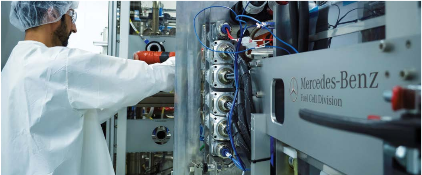
Factory acceptance test with operator at Mercedes Benz Fuel Cell Stack Production (Burnaby, British Columbia). Photo courtesy of Mercedes-Benz
