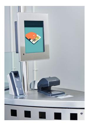
Management System (QMS), which involves the installation of tracking sensors and eGates. A network of tracking sensors in the ceiling anonymously tracks passenger movements in the queue and within the checkpoint, thereby reducing the number of times a boarding pass is scanned. eGates installed at the entrance of the checkpoint automatically validate boarding passes and Trusted Traveller credentials, and inform passengers of the next available screening line.
