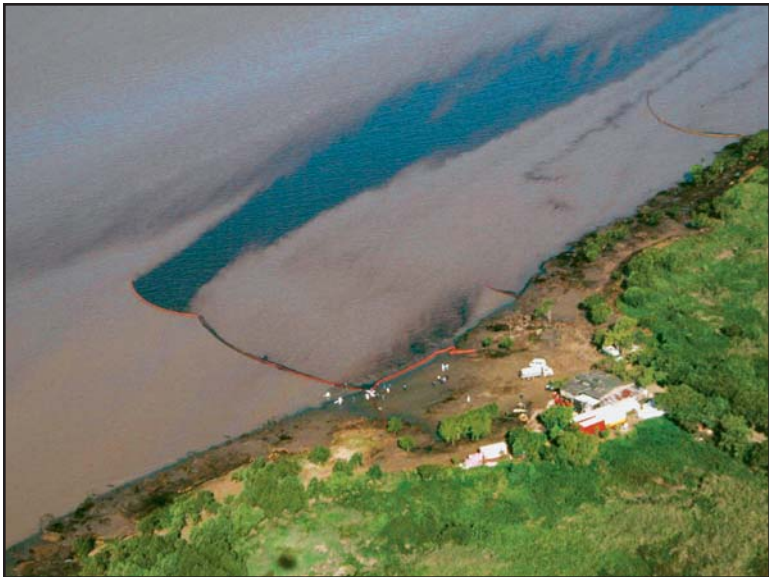
Figure 3.5 Oil is redirected towards the shoreline during the 1999 T/V Estrella Pampeana spill, River Plate, Argentina.
