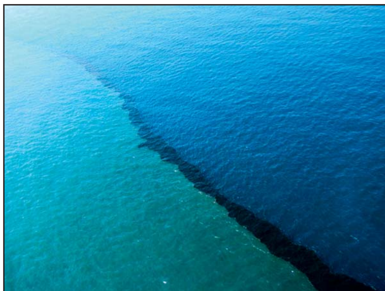
Figure 3.22 Oil is trapped at the density front. The turbid brackish water (left) is lighter in colour.
