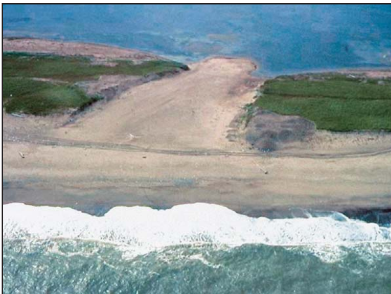
Figure 3.14 Low Overwash Channel on a Sand Barrier Beach with a Lagoon in the Backshore
