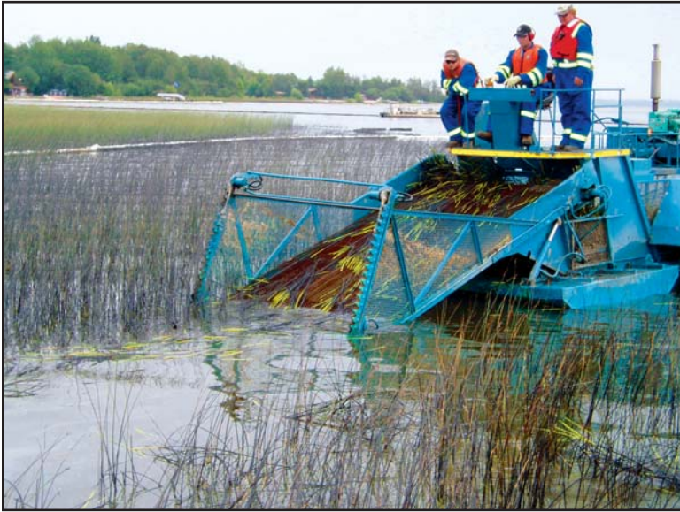
Figure 5.18 On-water Vegetation Cutting and Removal Using a Reed Harvester
