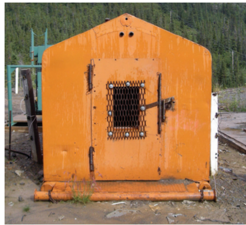
A metal waste storage container prevents access by wildlife.
