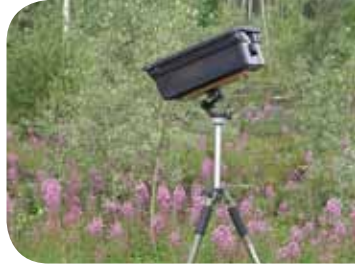
Bat detectors record ultrasonic bat calls nightly, for up to a week. (YG-T. Jung)
