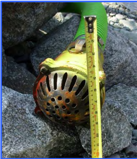
An example of a fish screen with holes that are too large.
