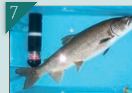
7 The receivers are now monitoring the movements of the tagged trout, recording all the 'pings' picked up from passing transmitters. We will visit each receiver and download the first year of data in summer 2014.
