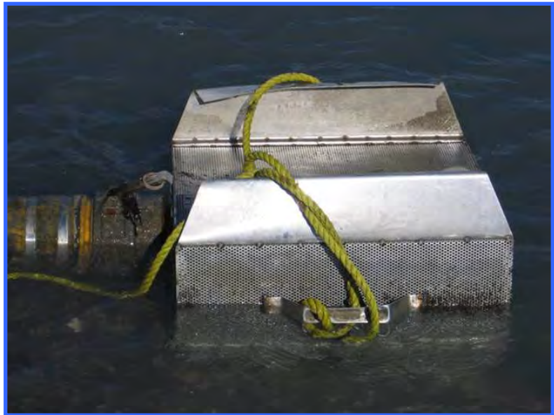
A typical fish screen for a 4" to 5" pump, fitted with correct screen size.
