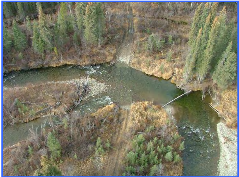
This type of stream fording is a thing of the past in Yukon, and never should have reached this state. There has obviously been many fordings over the years, leaving permanent marks in a fish-bearing stream. A temporary bridge should have been installed.
