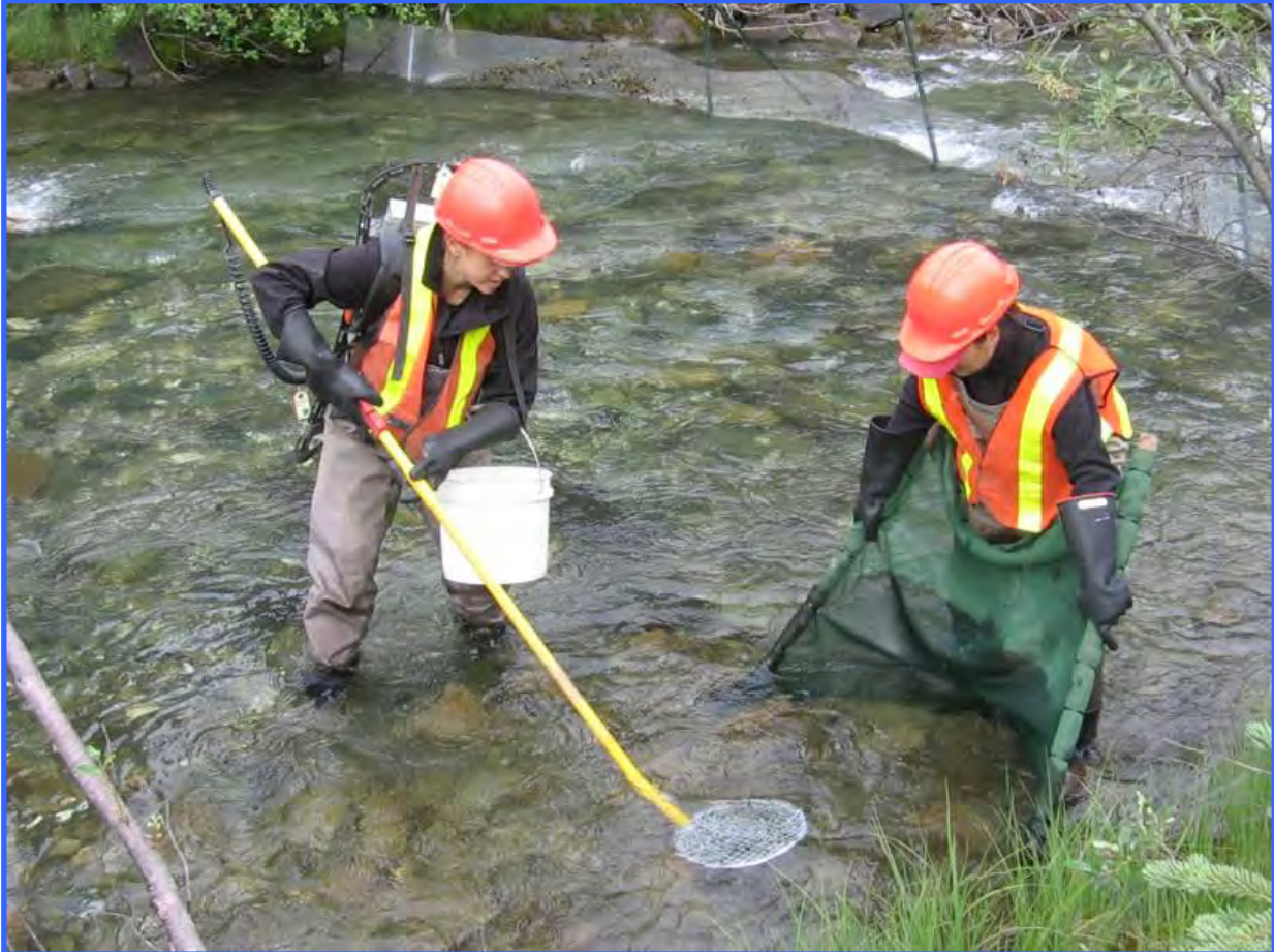
A fish salvage operation in progress. A section of the stream was netted off and fish were collected from the isolated area by means of electroshocking. The electroshocking unit is held on the back by the person on the left and the yellow pole is the shocking probe. The person on the right is helping retrieve the fish, which are only stunned for a fraction of a second so need to be caught quickly.
