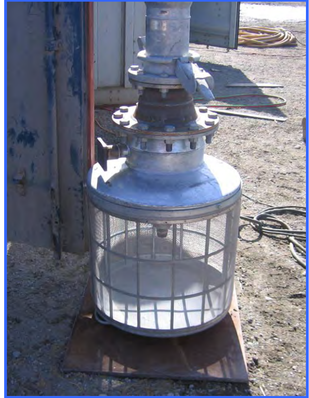
A very large fish screen for a high velocity 8" to 10" pump.
