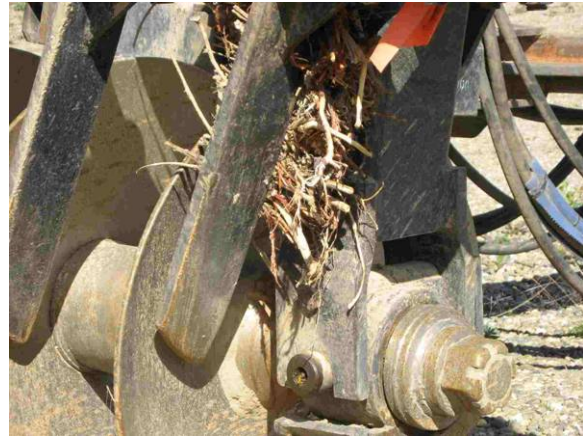
Figure 7b. Vegetation trapped in brush-cutting equipment. Seeds could easily be transported in this manner. Photo credit: M. Brunner
