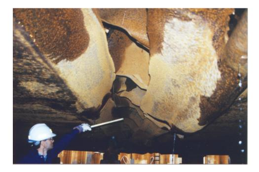
Post-occurrence calculations of the still water bending moment<sup>10,11</sup> (SWBM), imposed on the *Algowood* when partially loaded at Bruce Mines, were made to determine the magnitude and nature of bending stresses<sup>12</sup> incurred by the steel structure in way of the hull failure.
