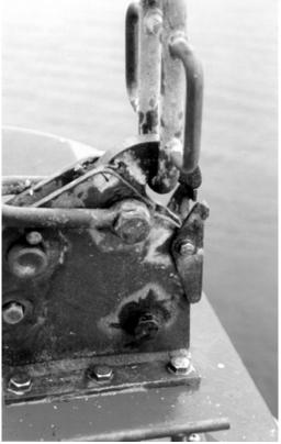
As long as the reset lever remains in a position where its cam prevents the blocking lever from rotating downward, the hook remains locked and can carry its portion of the designed weight of the lifeboat and its contents (see Photograph 10).
