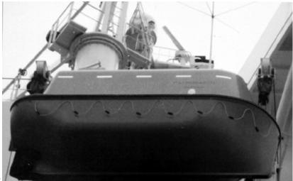
and 0.6 m high. It gives access to the after lifting hook, painter, and tow line. All three hatches are sealed by hinged covers that open inward, into the lifeboat.
