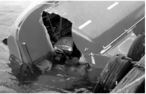
The impact with the water caused considerable damage to the stern of the lifeboat, with most of the damage concentrated around the canopy. The vertical panel was pushed inward, and the glass-reinforced plastic was
