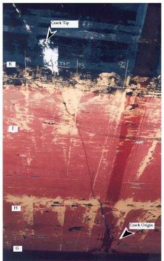
The fracture had not grown appreciably since the initial discovery, as a crack-arresting hole had been drilled at the crack tip to limit the growth of the fracture.
