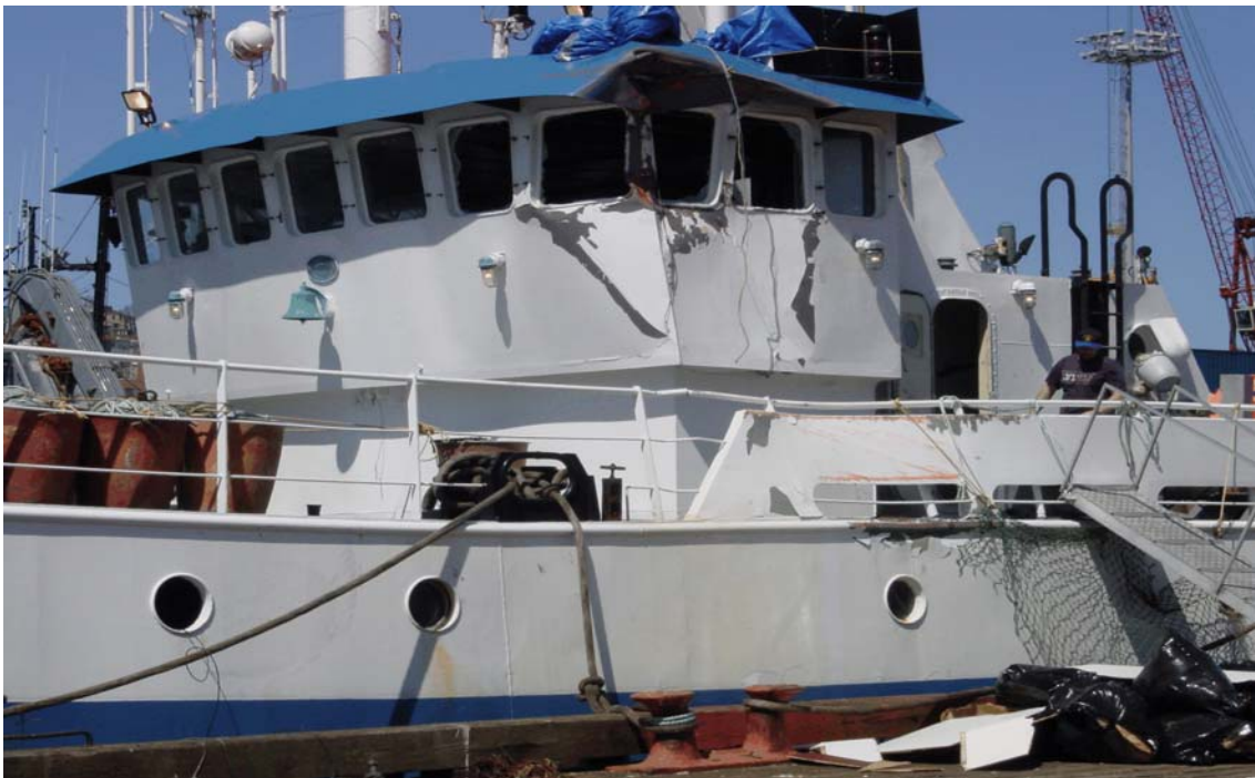
Photo 3. The damaged superstructure of the Genny and Doug
