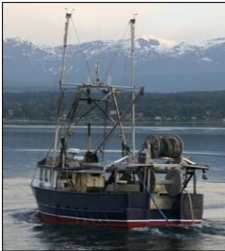
Photo 4. Stern view showing additional trawl, A-frame rigging, trawl stanchion
