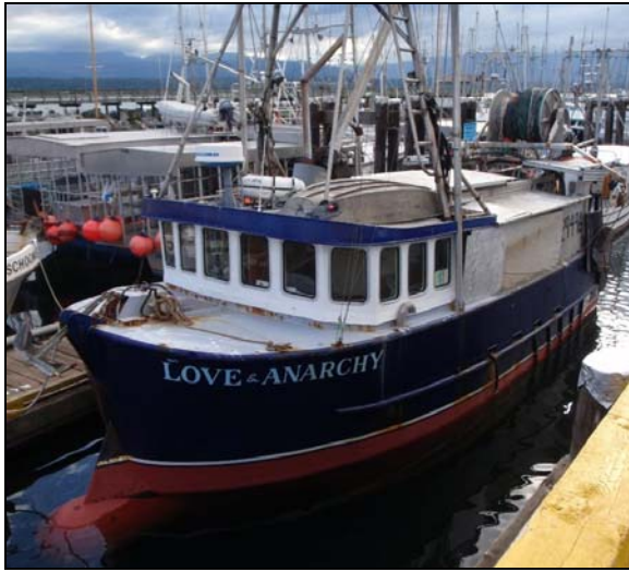
Photo 2. Front view showing aluminum canopy over working deck
