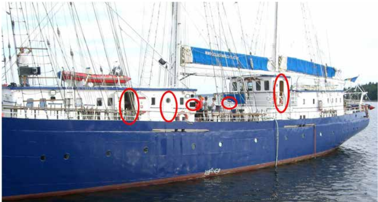
Photo 3. Some critical port side openings
