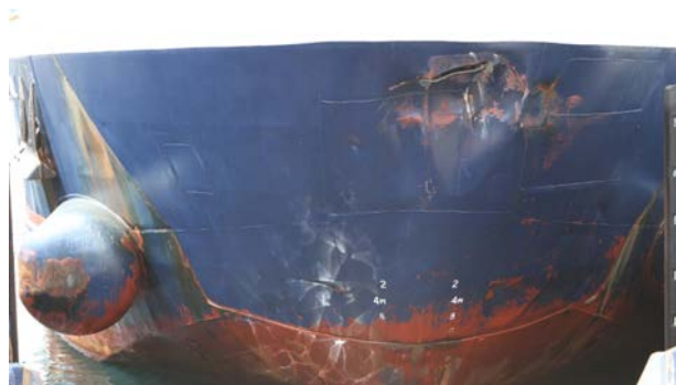
Photo 2. Damage to bow visor
