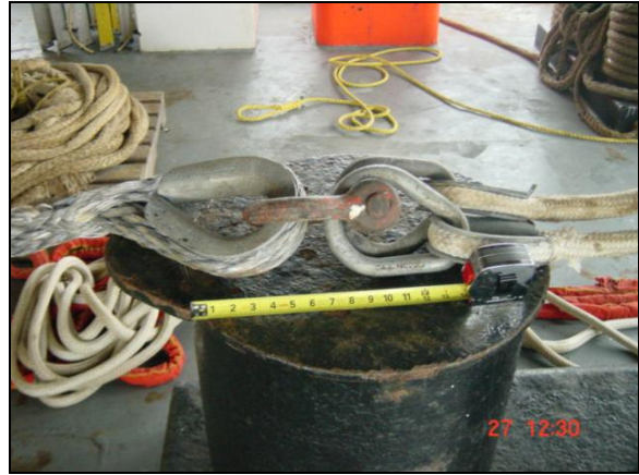
Photo 3. Towline to bridle connection arrangement
