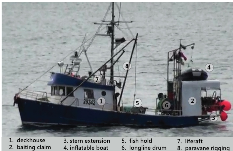
Photo 1. The Pacific Siren's general arrangement.
