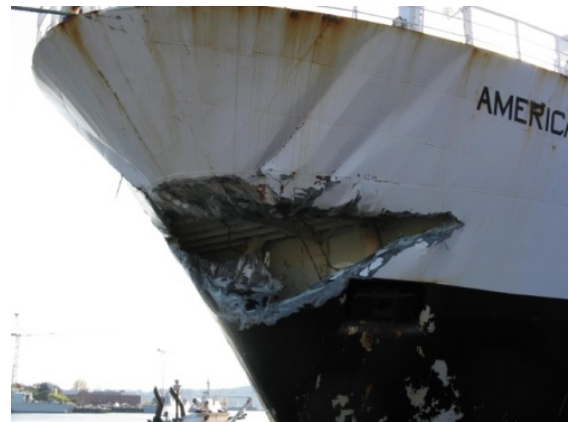
Photo 2. American Dynasty damage
