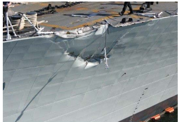
Photo 3. Damage to the HMCS Winnipeg's port side
