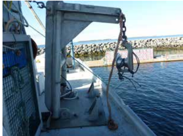
Photo 3. Overhead block in raised position
