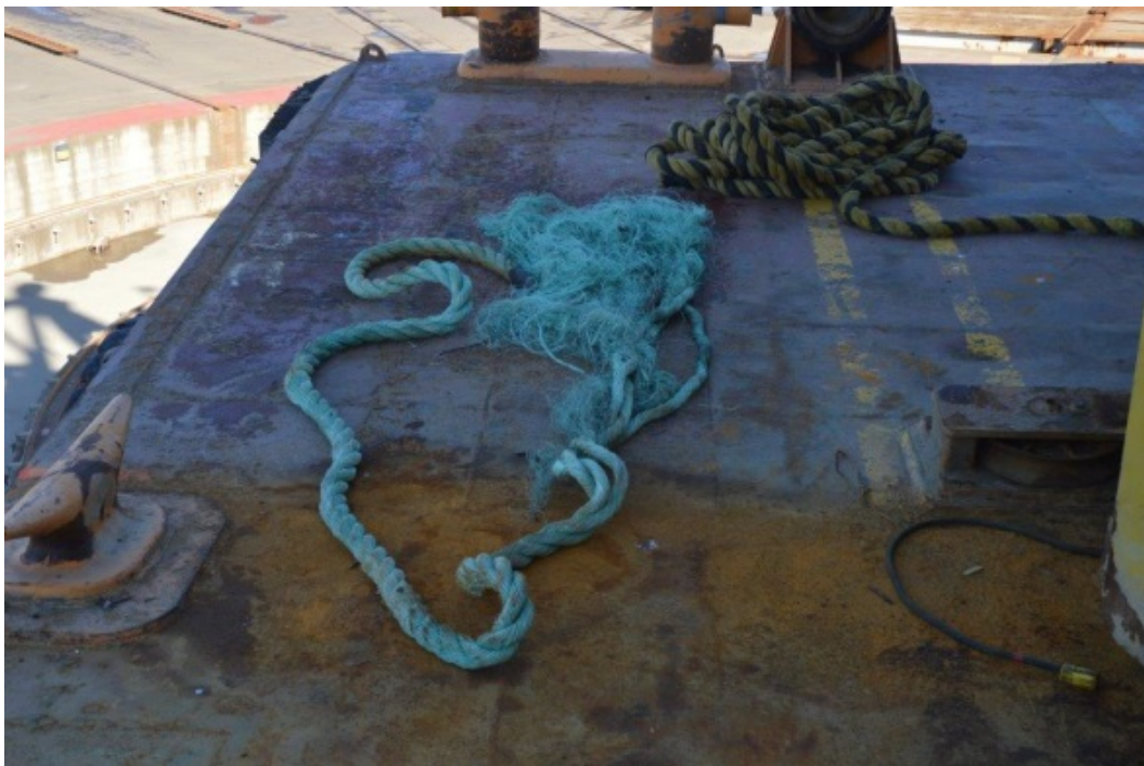
Parted 48 mm copolymer rope with frayed end on the HM Tacoma
