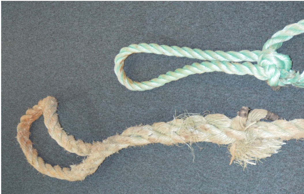
Parted 48 mm copolymer rope with frayed end on the HM Tacoma
