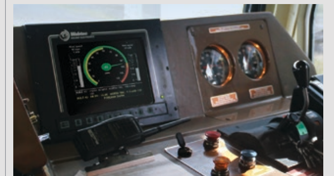
RIGHT: GPS Control System panel installed on our locomotives
