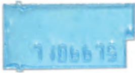
FIGURE 9. A solid-state nuclear track detector that uses CR-39 technology.
