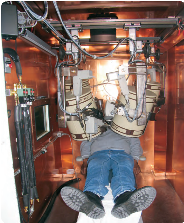
FIGURE 11. A typical lung counter. The device shown is used by Health Canada at its Radiation Protection Bureau in Ottawa.
