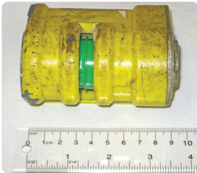
FIGURE 14: A personal alpha dosimeter.
