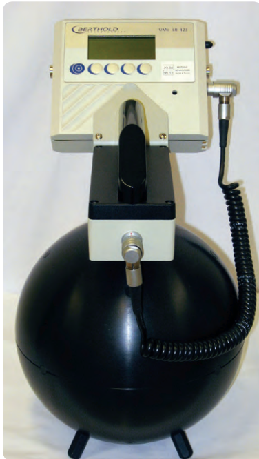
FIGURE 10. A portable neutron survey meter.
