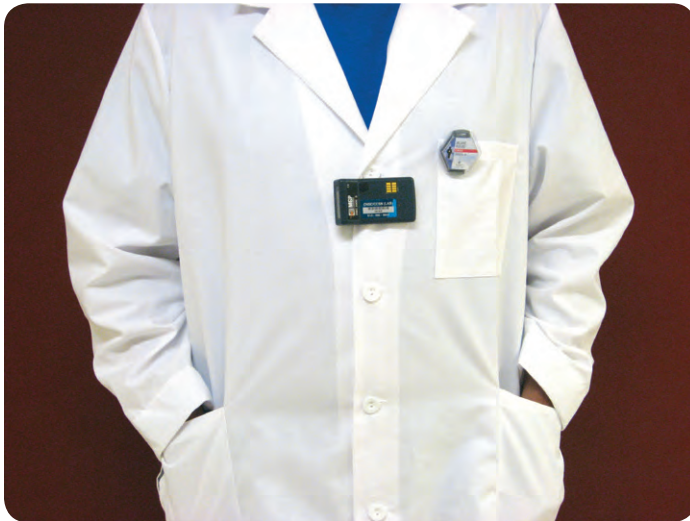
FIGURE 7. A direct reading dosimeter and an optically stimulated luminescence dosimeter, worn on the front torso.
