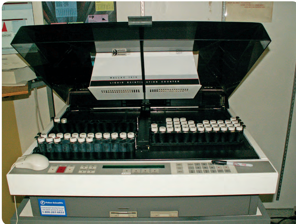
FIGURE 13. A liquid scintillation analyzer.
