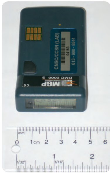
FIGURE 6. A direct reading dosimeter.
