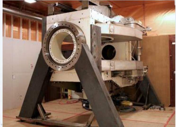
Prototype MR-Linac (source: mp.med.ualberta.ca)
