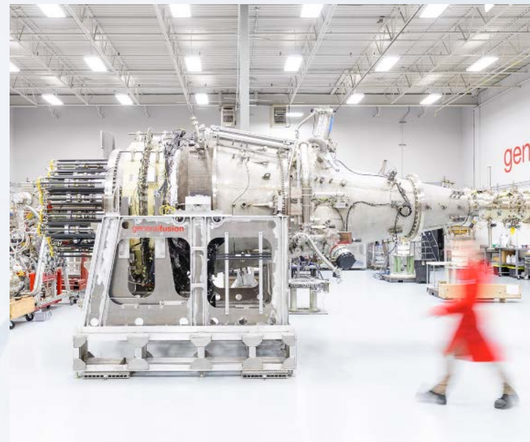
Plasma injector (source: generalfusion.com )
