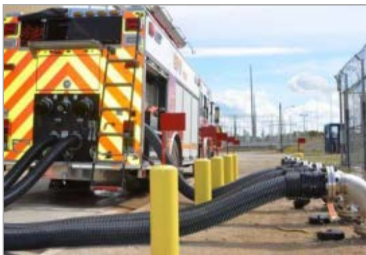
Bruce Power Fire trucks provide cooling water. New emergency water pumping equipment procured and on site.
