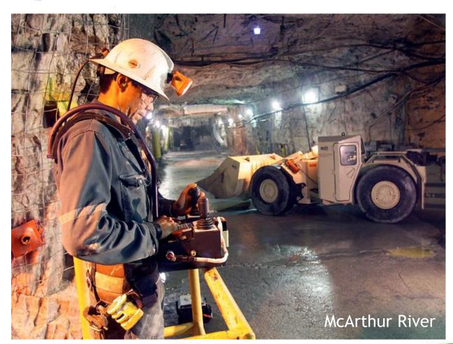
A person operates a scoop tram remotely to scoop up the muck.
