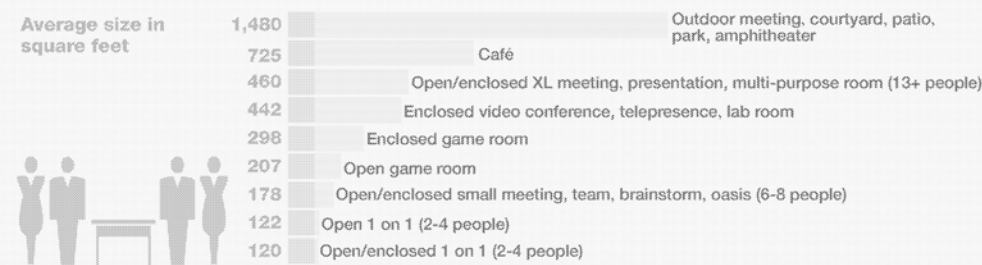
Figure 7. Collaborative spaces used in distributed work range in size from outdoor spaces (1,480 square feet) to enclosed “thinkspace” for two people, which can be as small as 116 square feet. Note: Data presented show the average square footage for all participants, for each space type.
