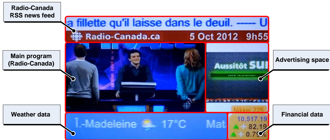
FIGURE 3 - Mobile DTV screenshot showing metadata features (Montreal mobile DTV service shown)
