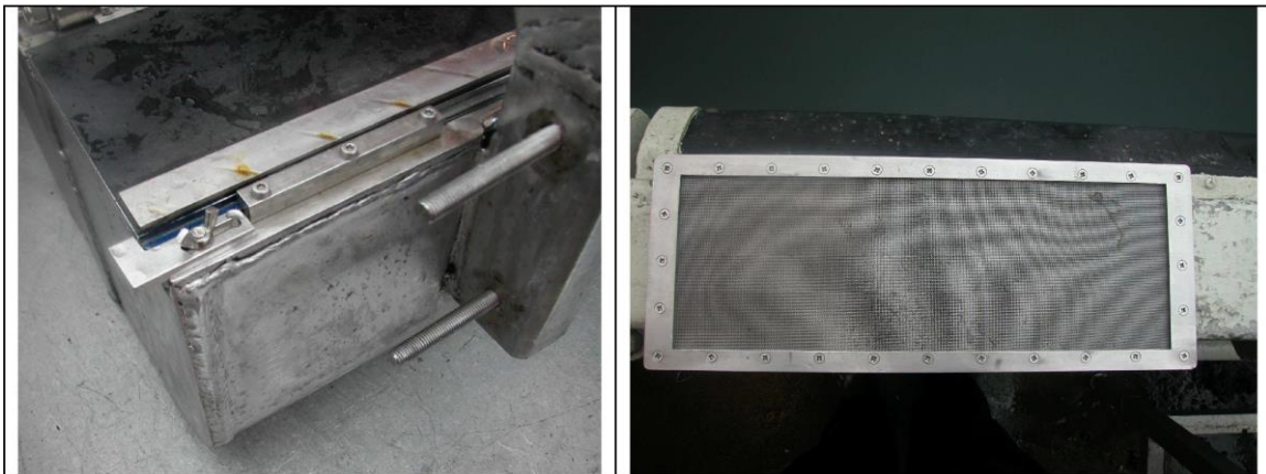
Left side: locking mechanism for the screen. Right side: screen with 0,5 mm mesh
