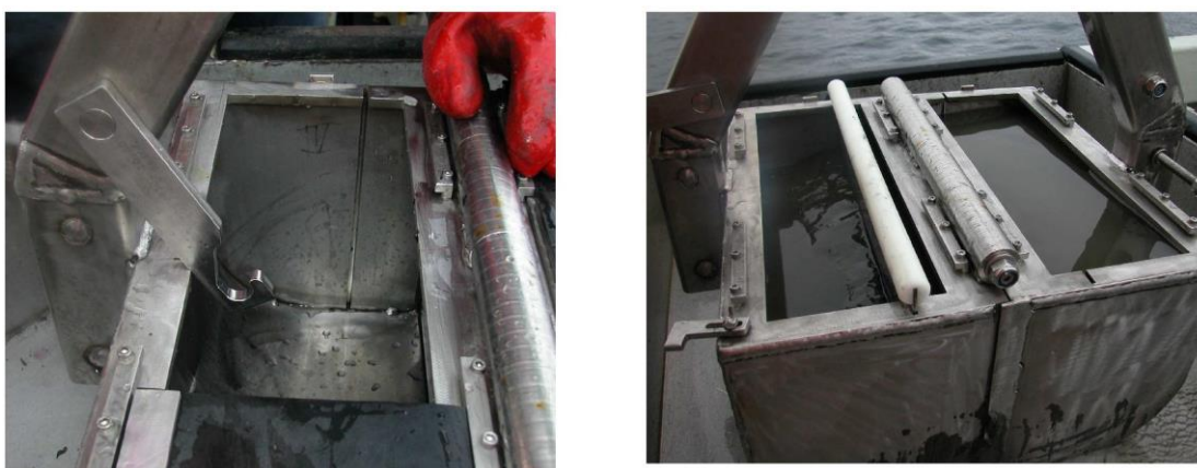
Figure 2-6. Illustrations of sliding tracks and grab sampler with divider
