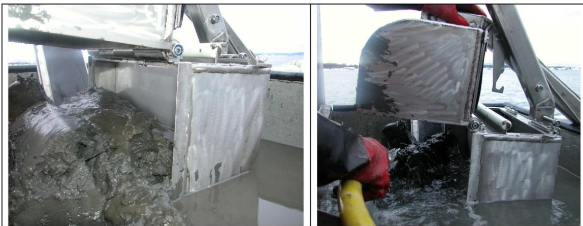
The divider splits the sample in two so that samples can be processed independent of each other.
